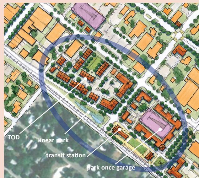
Conceptual drawing of potential mixed-use, transit-oriented development surrounding new rail station with added green space, "park once" garage, new retail, housing, and office space; located along Hill Ave between Coll and Garden, transforming under-utilized industrial lot in Downtown for economic development opportunities.
