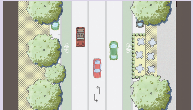
Site plan shows movable tables and planters in the parking space to extend cafe dining area. Planters create buffer to traffic and can easily be removed if parking space is needed for other use.
