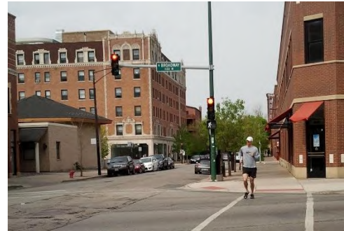
LPIs allow people walking to enter the crosswalk before vehicles are given the green phase.
