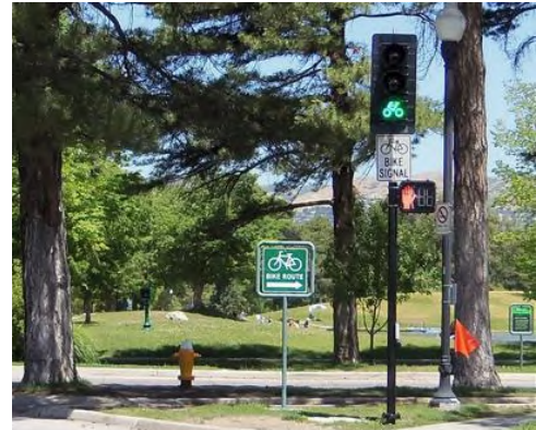
An intersection with bicycle signals may reduce stress and delays for a crossing bicyclist, and discourage illegal and unsafe crossing maneuvers.
