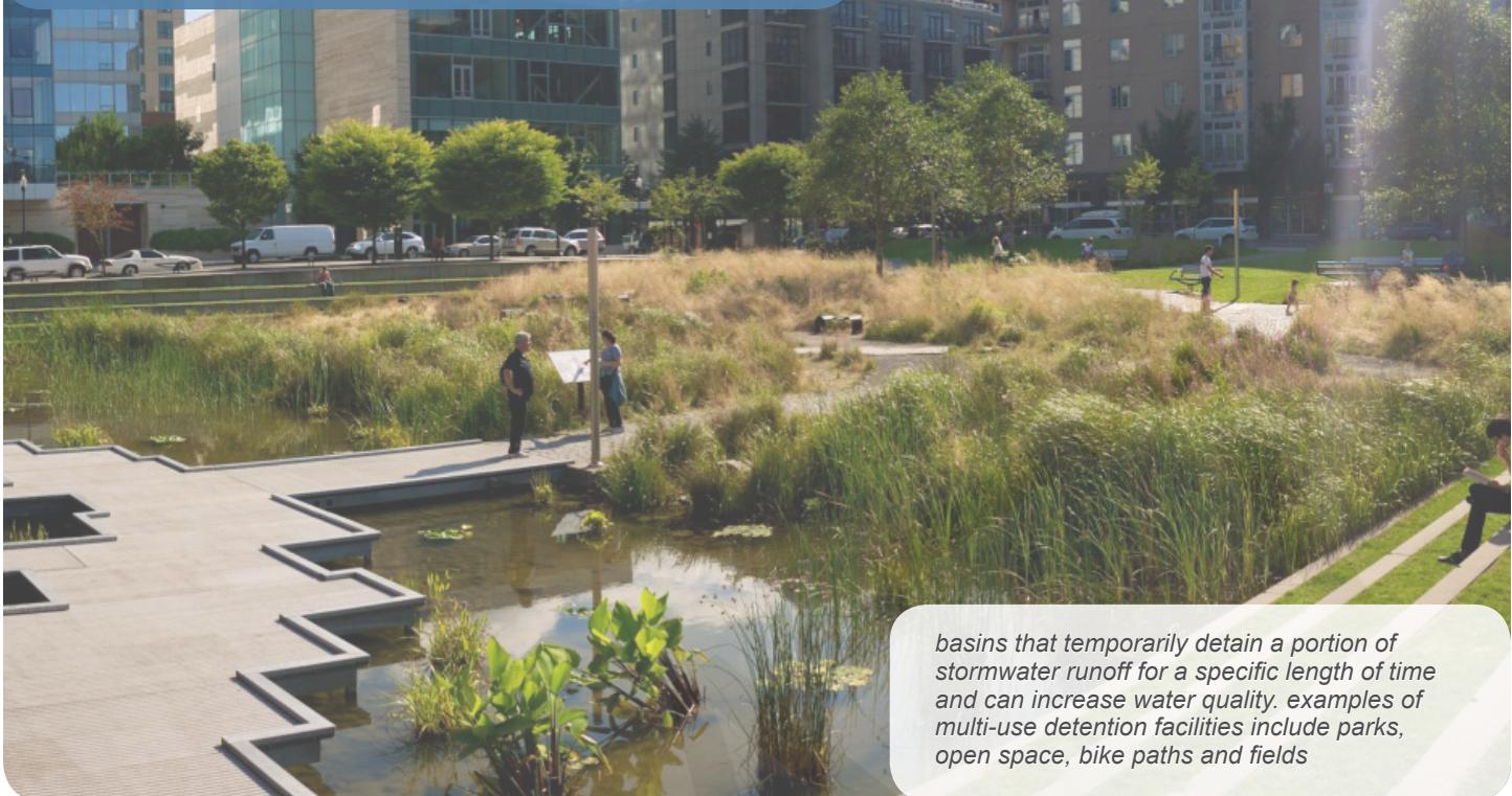
*basins that temporarily detain a portion of stormwater runoff for a specific length of time and can increase water quality. Examples of multi-use detention facilities include parks, open space, bike paths and fields*
